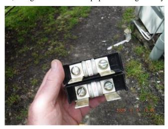
The assembly of panels is damaged in several places, and we recommend repair or replacement by a qualified electrician. The panels also appear to be worn past a reasonable point of repair and maintenance and we suggest replacement of the entire assembly.
