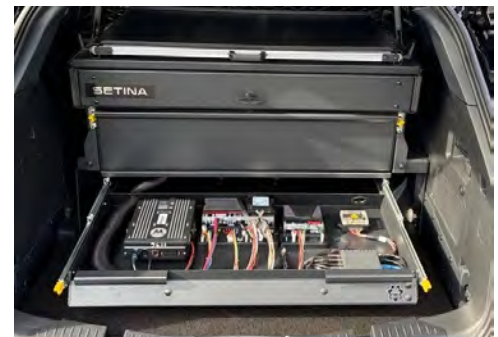
Behind the scenes: radio and power equipment housed in a secure rear cargo drawer.
