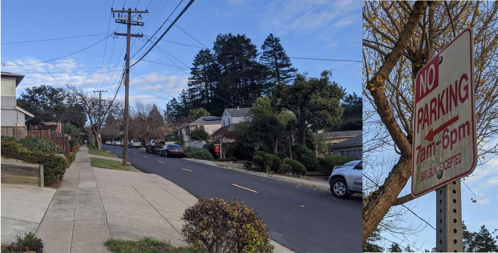
Figure 10: Beloit Avenue, looking east between Trinity and Colgate Avenues, showing extensive on-street parking, narrowing to a minimum of 16 feet and forcing multiple segments of one-way traffic. Several parking spots are already time-restricted (see right) to allow AC Transit buses to make a left turn off of Trinity Avenue during service hours.
