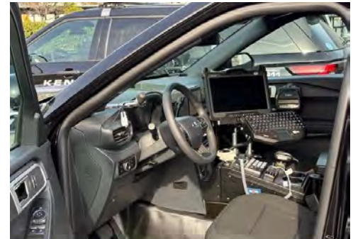
The driver's workstation: mounted Getac computer, keyboard, and console controls within easy reach.
